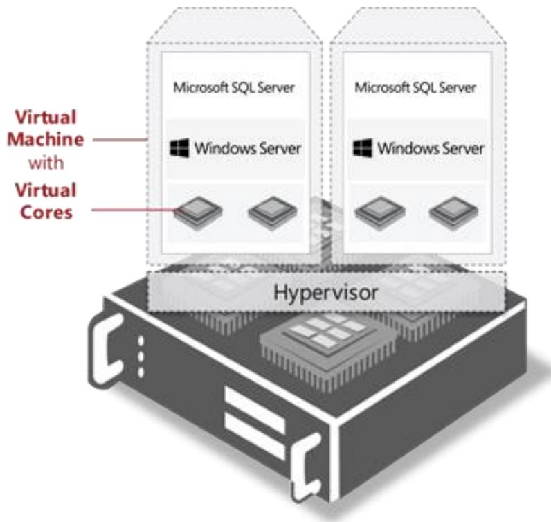
Figure 4: Virtual Machine (VM) using virtual cores
